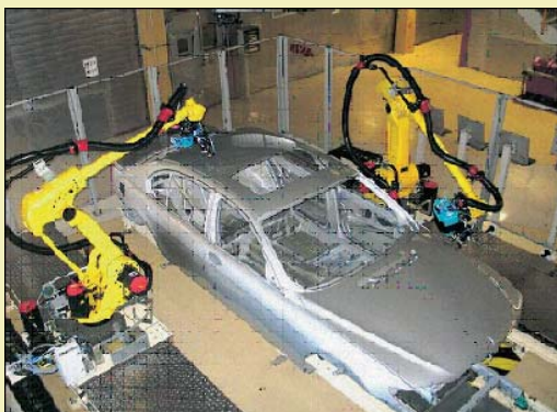
◀ Robots measure the painted car bodies, ensuring reproducible results
