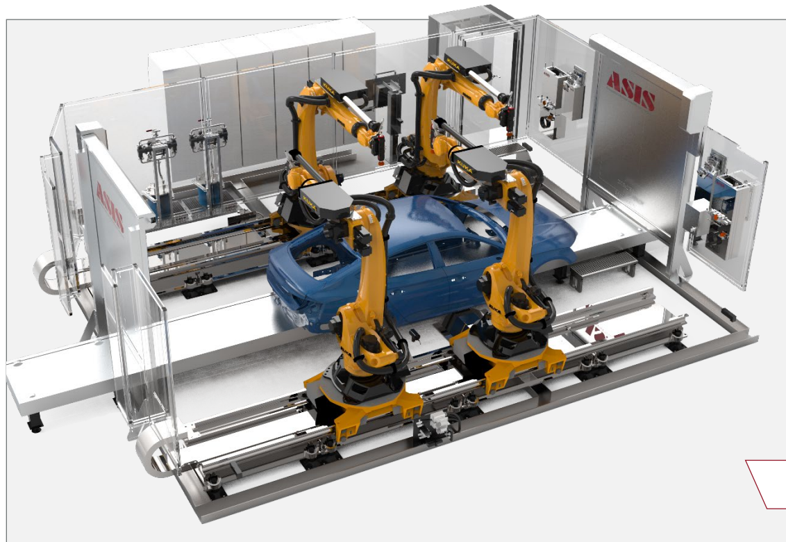
Automatic finish cell with polishing & sanding
