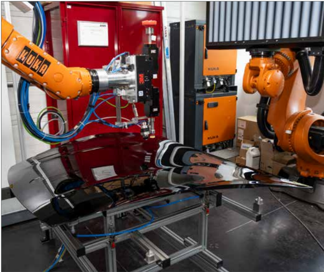
Fully equipped automatic finish test cell with defect detection
