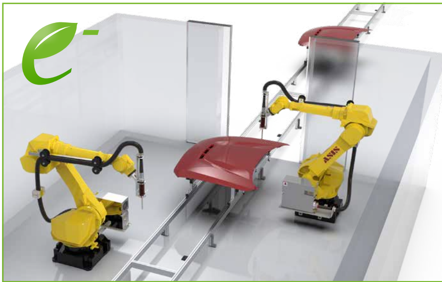
The combination with an industrial robot enables the integration into the painting line
