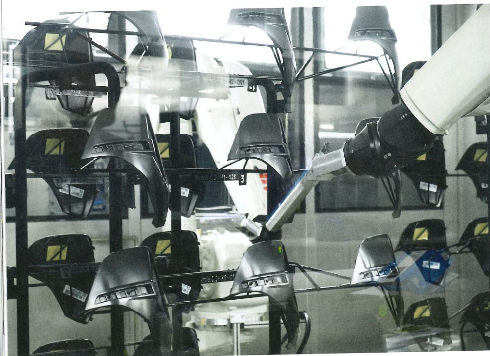
The flame treatment activates the surface of plastic parts and ensures increased paint adhesion.
